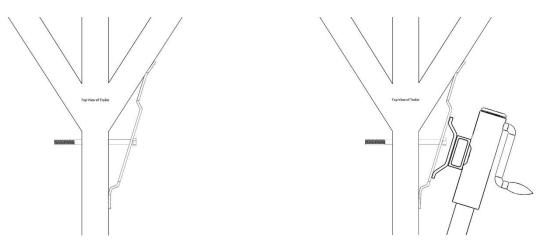
**STEP 9:** Mount the jack stand with provided 7/16<sup>th</sup> bolts and lock nuts. Tighten everything and rotate positions of shield and jack stand to confirm all clearances.
