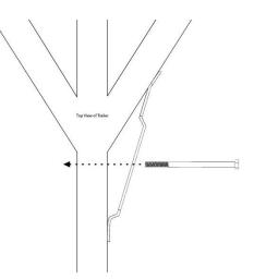
**STEP 7:** Install jack stand relocation bracket as shown. The top edge of the plate MUST BE FLUSH with the top edge of the trailer. This relocation of the jack stand will give you clearance to use the jack stand and the shield. Note: Jack stand must be in the down position when using the ramp. Mount jack stand plate by pre-drilling (10) <sup>1</sup>/<sub>4</sub>" holes into the plate as shown. Use the 10 provided self tapping screws to mount plate to the trailer.
