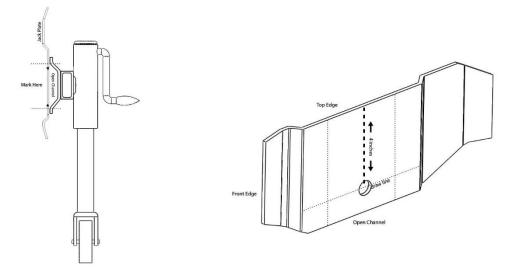
**STEP 6:** To mount the bolt through trailer neck, mount the plate with one screw on each side. Drill through the plate and mark on the trailer neck where the bolt will go. Remove the plate and drill through the trailer neck through the opposite side. Position the drill so that the bit is 90 degrees to the trailer neck.
